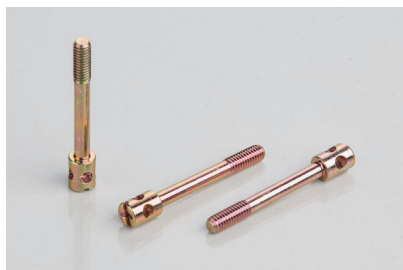
Four-Hole Combined Slot Seal Screw M4×31×10 Low Carbon Steel Hexavalent Iridescent Zinc Plated
