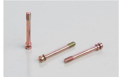
Export Special Break-off Slotted Anti-reverse Screw M4×32×8 Low Carbon Steel Hexavalent Iridescent Zinc Plated
