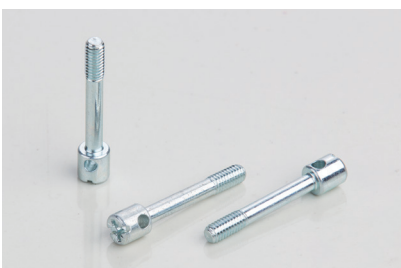
Export Special PZ Slot Cylinder Head Single-Hole Seal Screw M4×20×8 Low Carbon Steel Trivalent Iridescent Zinc Plated
