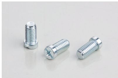
Export Special Cylinder Head Combined Slot Torque Off Seal Screw M8×15 Medium Carbon Steel Trivalent Iridescent Zinc Plated
