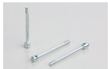
Export Special PZ Slot Cylinder Head Single-Hole Seal Screw M4×45×8 Low Carbon Steel Trivalent Iridescent Zinc Plated
