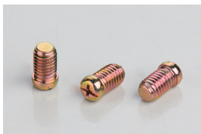
Pan Head Combined Slot Torque Off Seal Screw M8×12 Low Carbon Steel Hexavalent Iridescent Zinc Plated
