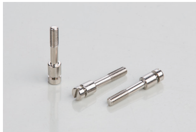
Export Special Break-off Slotted Anti-reverse Screw M4×20×10 H62 Brass Nickel Plated
