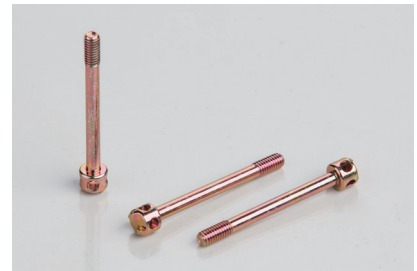
S-Type Slotted Anti-reverse Seal Screw M4×40×8 Low Carbon Steel Hexavalent Iridescent Zinc Plated
