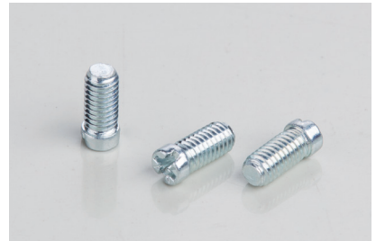
Export Special Cylinder Head PZ Drive Torque Off Seal Screw M5×12 Medium Carbon Steel Trivalent Iridescent Zinc Plated
