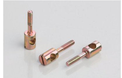
Cylinder Head Slotted Large Head Seal Screw M4×22 Low Carbon Steel Hexavalent Iridescent Zinc Plated
