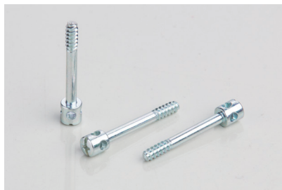
Export Special Round Head Four-Hole Seal Screw ST4×31×8 Low Carbon Steel Trivalent Iridescent Zinc Plated
