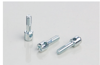
Export Special PZ Slot Cylinder Head Single-Hole Seal Screw M4×14×8 Low Carbon Steel Trivalent Iridescent Zinc Plated
